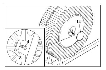
2. Pry the Access Cover (14) off the left side shield. Loosen the M8 Washer Nuts (4). To tighten the chain, turn the M6 Adjustment Nuts (8) clockwise; to loosen the chain, turn the Adjust-ment Nuts counterclockwise. Make sure that the fan is straight, tighten the Fan Nuts and reattach the Access Covers.
